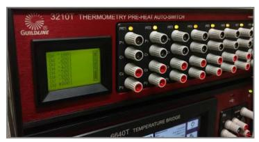
single or multiple tests can be initiated while the Bridge is unattended. All user **definable test variables**, such as excitation current, pre-heat current, measurement speed, reversal rate etc can be **programmed on a per test basis**, giving the **users full control and flexibility** in conducting well designed measurements, and for calibrating temperature probes.
