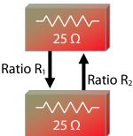
The 1:1 measurement ratio can be easily calibrated and verified by interchange measurement tests using two stable standard resistors of same nominal values, as illustrated by the block diagram to the right. Bridge 1:1 measurement ratio error  $e_i$  (in ppm) is calculated using the following formula:
